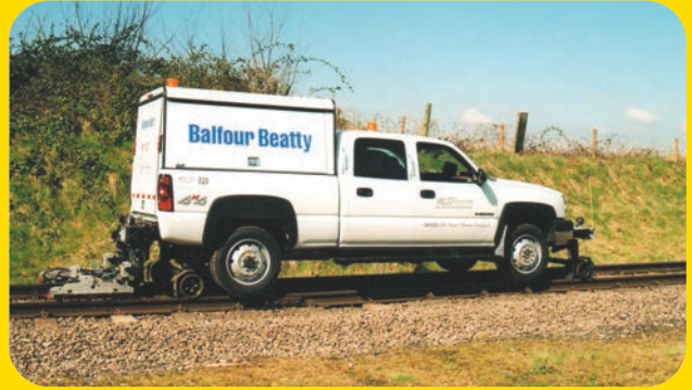
High-speed rail crack detection.
