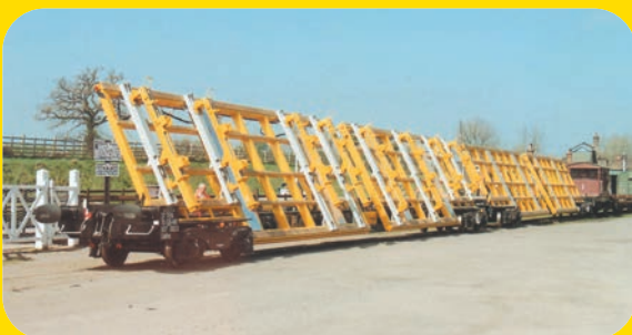
Tilting table wagon for points and crossings.
